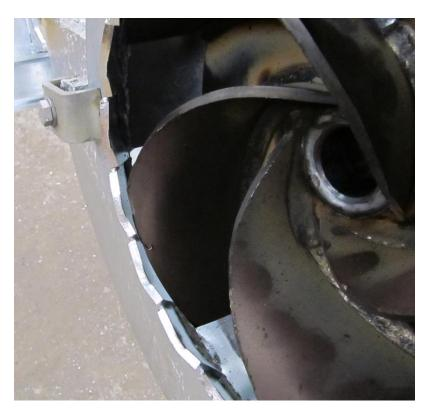
In order to maintain good cutting productivity, distance between the impeller and the cutter should be 2-3 mm. The distance is checked at least once per season or after 40 hours. If the distance is too small, an impact may occur, causing vibration. Too large distance will cause loss of power.
