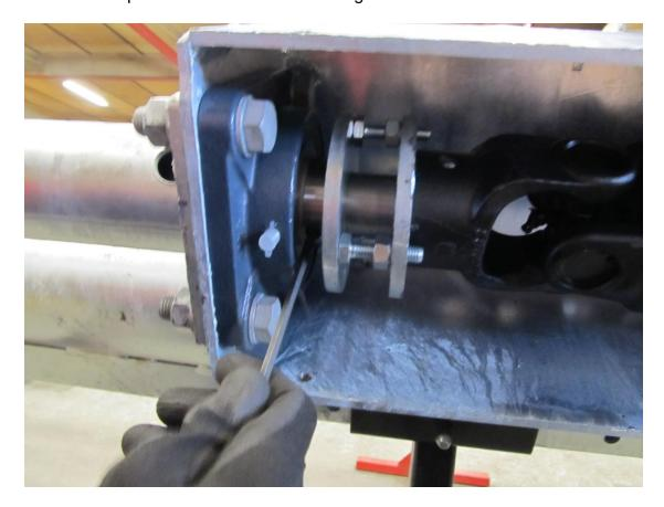
3. Adjust the distance in the pump housing by adjusting the distance washers between the bearing and the universal joint. By reducing the distance between washers, the universal joint will be moved down towards the bearing and the distance between the impeller and the cutter will decrease. It is important to check if the distance between three adjustment screws is the same.
